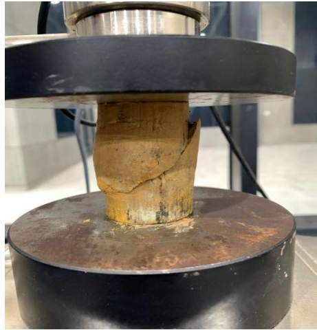
Gambar 6. Pengujian Kuat Tekan Bebas ( Unconfined Compression Strength Test )
